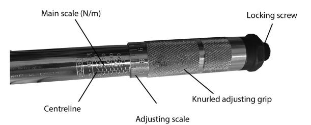
Hold the torque wrench in your left hand (if right handed) so that the required scale - foot/pounds or Newton/metres - is uppermost and visible.
